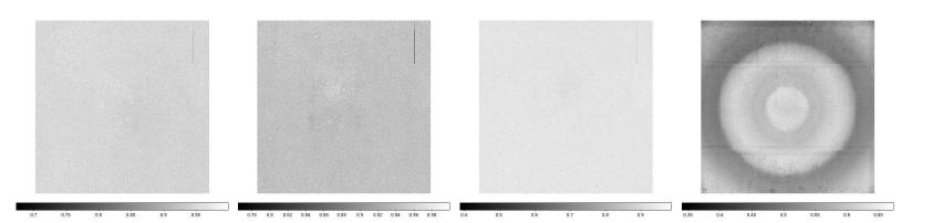
i' filter observed with LEDs at 735 nm, 750 nm, 810 nm
