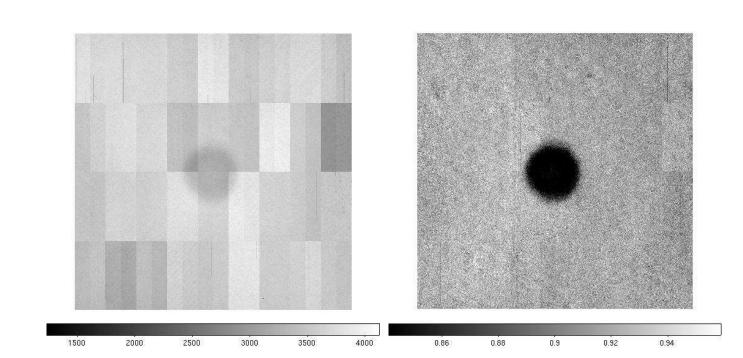
A 480 nm LED illuminating the mosaic with the filter g' in front of the CCDs (left). By making the ratio of that image with one taken without any filter, we obtain the g' filter transmission (right), showing an inefficiency of 10% in the center.
