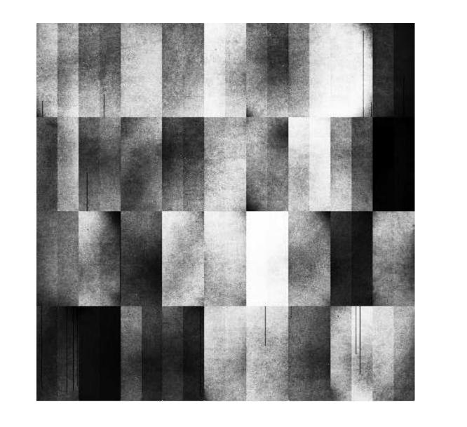
Illumination with a 850 nm LED, without filters (plotted for maximum contrast). The difference in responses at the level of the half-CCDs are due to the different gains of the readout amplifiers. The inhomogeneities of CCD efficiencies are also detected.
