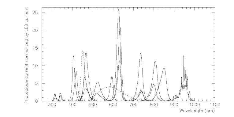
Spectra of the 24 LEDs selected for the calibrated LED source, and of the 'white' LED used for the artificial planet
