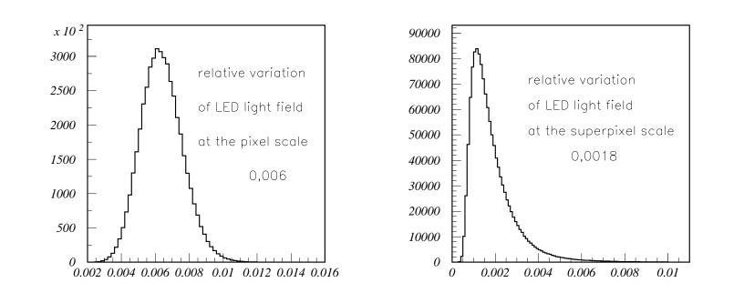
Stability of the LED illumination at each pixel/superpixel, evaluated on 16 successive shots in identical conditions.
