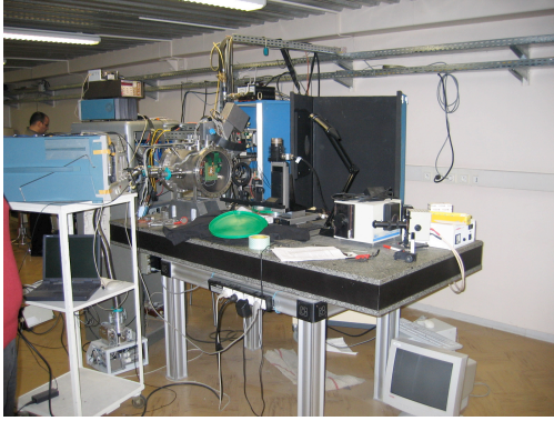
Figure 2.14: First test bench in Paris. One can see an X,Y motion device in front of a tube connected to a cryostat in which is a “focal plane” with CCD and Photodiodes.
