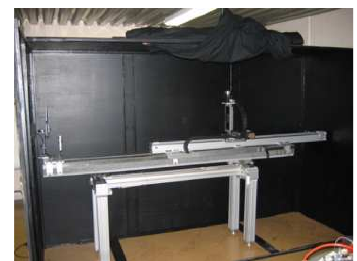
Figure 6: Test bench inside a black box for 3D calibration of the LED source.
