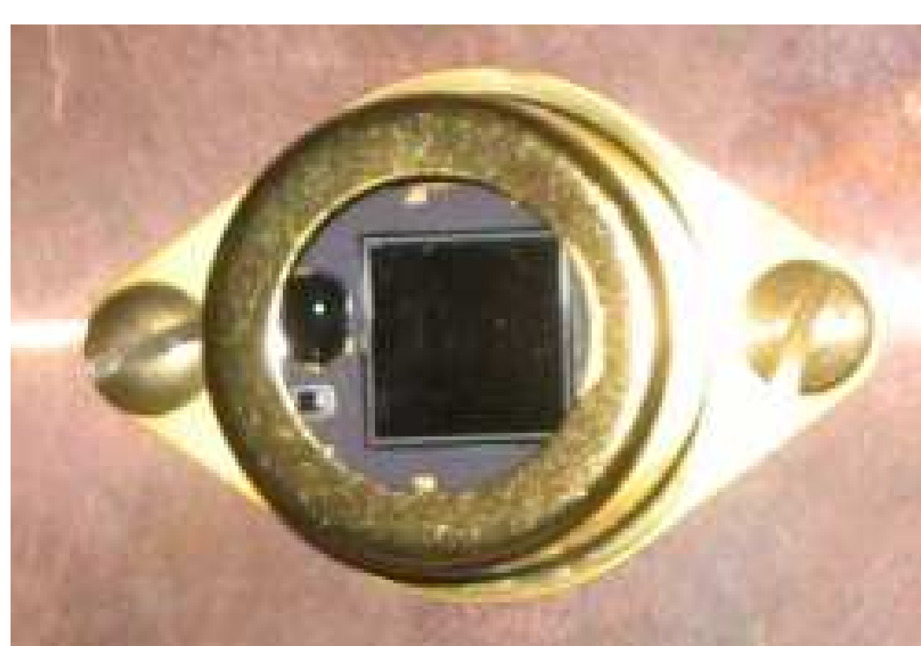
Figure 5: The Hamamatsu S3477 photodiode (including a Peltier cooler).
