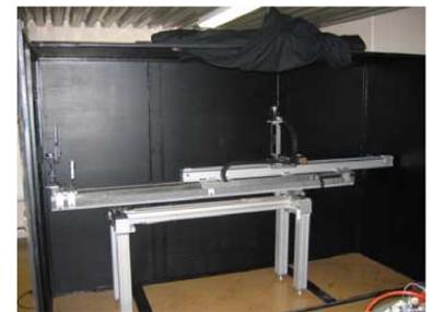
Figure 6: Test bench inside a black box for 3D calibration of the LED source.
