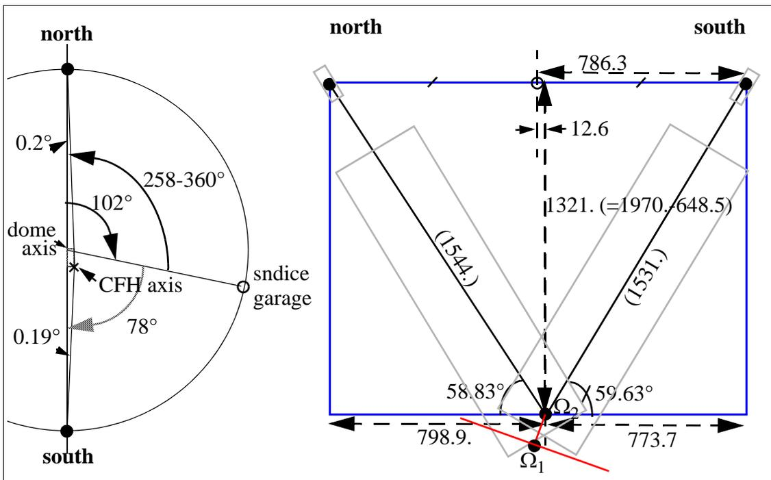
**Figure 6:** Schematics of the surveying of SNDICE using CFHT as a theodolite compared with the laser survey of Figure 15. The radius of SNDICE «orbit» is  $786.3=(798.9+773.7)/2$  compared to laser's 796. cm. A 12.6 cm southward offset (and 2.7 cm eastward) of the telescope axis relative to the dome axis reproduce angular measurement mismatches (see left drawing).
