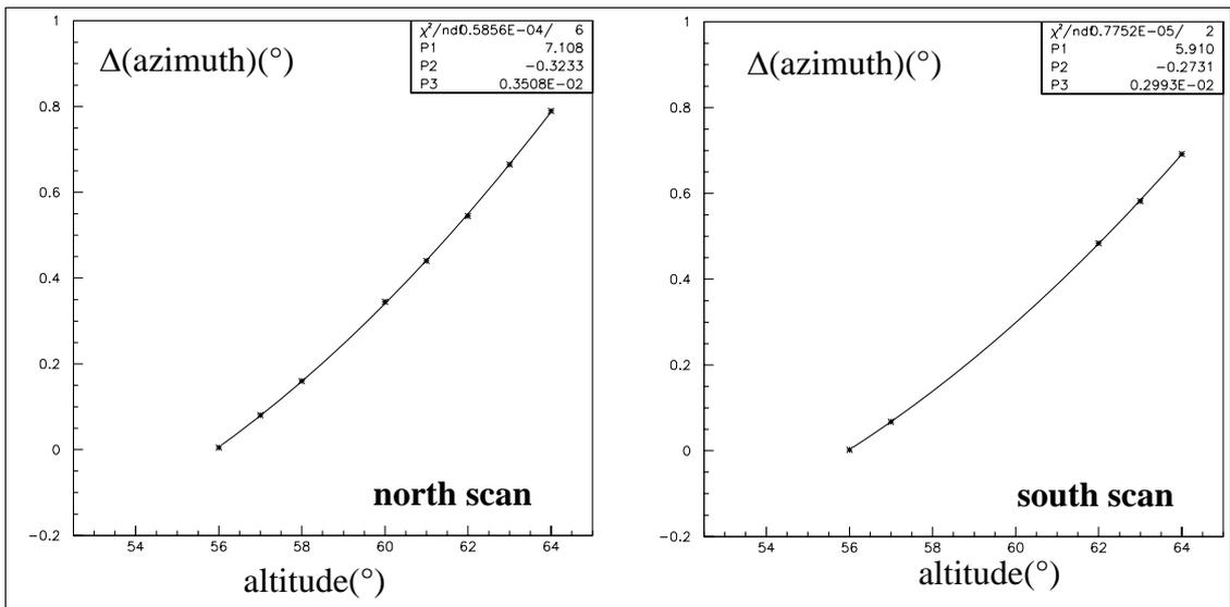
**Figure 4:** The fit of the difference between SNDICE azimuth and CFHT's as a function of altitude yields a large relative angle of vertical planes from both systems. This seems in contradiction with the fact that horizontal and vertical motors are hold together by a right angle bracket.
