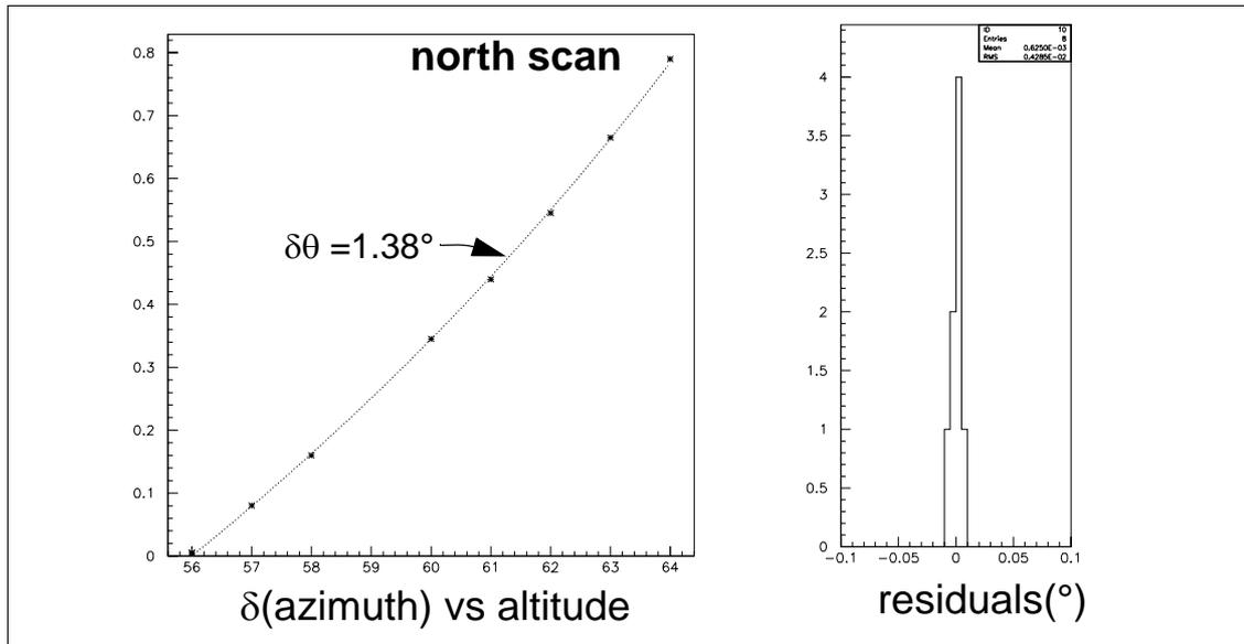
**Figure 8:** Fit of the vertical skew of Figure 4 with the analytical single parameter ( $\delta\theta$ ) formula taken from spherical trigonometry. Note that the effect of a  $\delta\theta=1.38^\circ$  skew angle is a  $5.7^\circ$  inclination of the vertical axis in the tangent reference system, because of the high altitude of SNDICE ( $60^\circ$ ).
