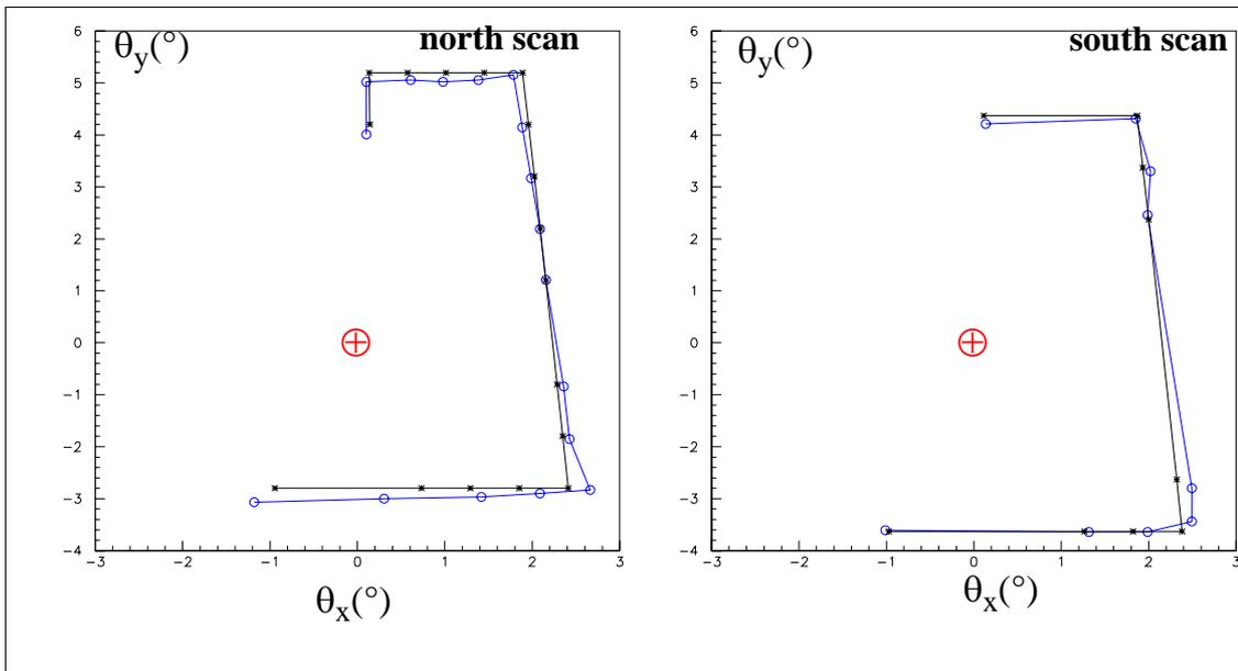
**Figure 7:** For the north and the south AP scans, the angular coordinates of the telescope in the local tangent SNDICE system (○) are compared to the angle of incidence (\*) on the focal plane determined using the double reflection AP spot. The origin of coordinates (⊕) corresponds to the normal incidence (virtual ray joining the center of the mirror to SNDICE AP led -not physical since it traverses the camera).
