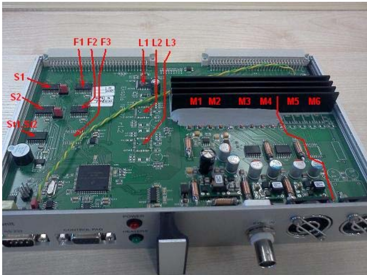
Figure 1 OPG driver board. Depending on a number of controllers in specific OPG's, some PCB components shown above may be not included.
