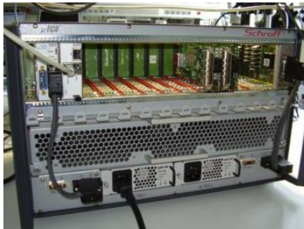
FIG. 31: Picture of a micro-TCA crate containing DAQ boards with 32 ADC channels/board as developed in 2010.
