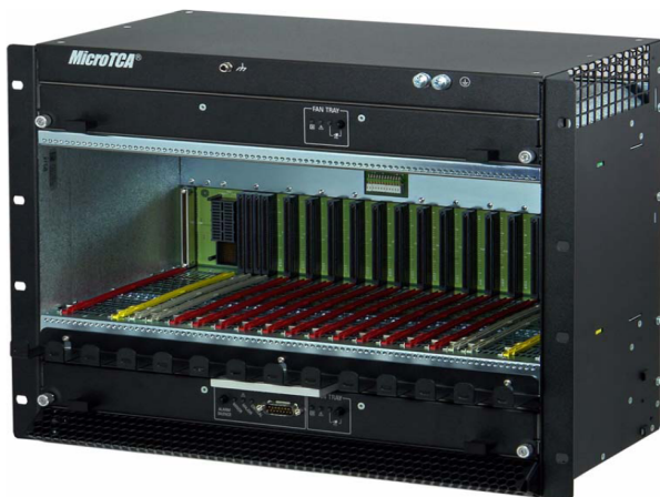
FIG. 39: Left: picture of the Schroff 11850-015 8U shelf. Right: sketch of crates implementation on the top layer of the prototype detector. Each red box features a crate. The inter-chimney distance, of the order of 1 meter, allows this type of crate disposal which minimizes the constraints on cables lengths.
