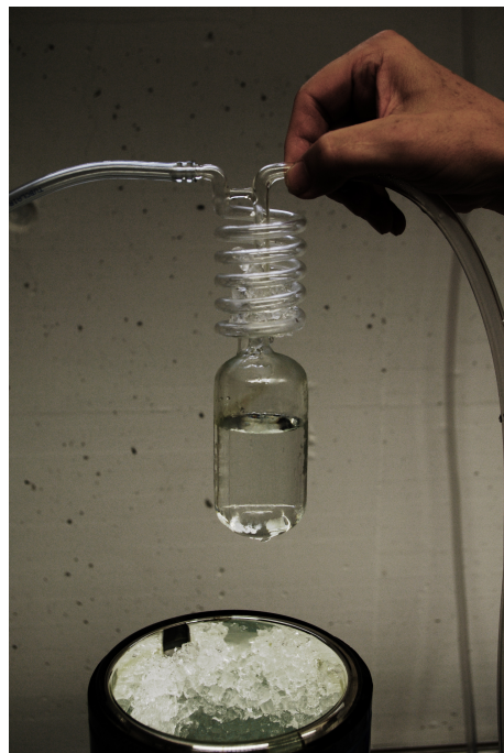
FIG. 58: Collected water from regeneration of a copper cartridge.
