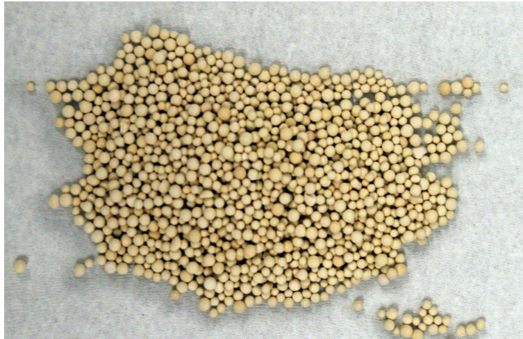
FIG. 56: Molecular sieve ZEOCHEM 3A ® grains before inserting them in the regeneration cartridge. Each grain has a diameter of about 2 mm.
