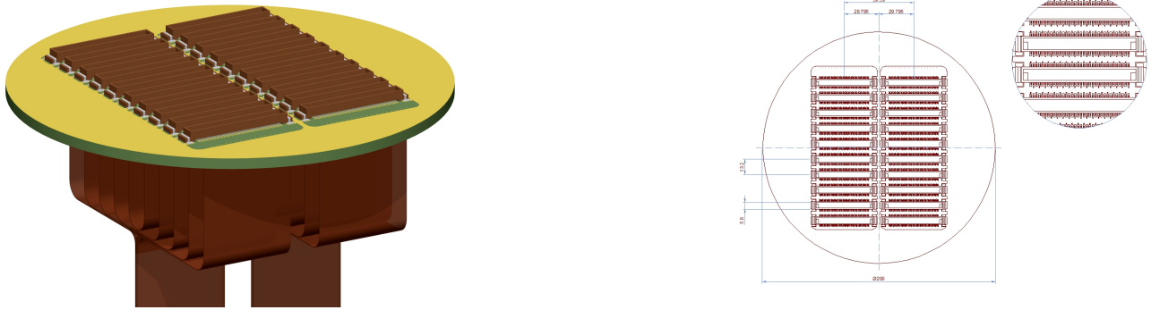
FIG. 43: Signal feedthrough and connectors from the CRP (left) 3D view (right) 2D top view.
