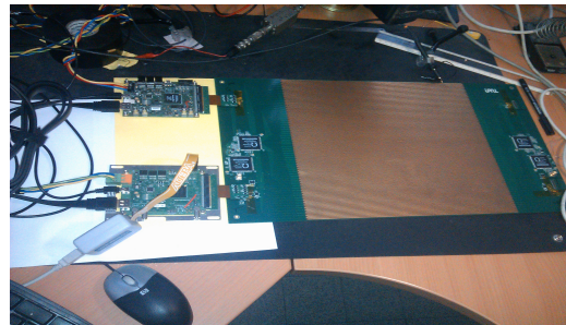
RE1/1 chamber built and successfully tested using electronics developed for ILC
