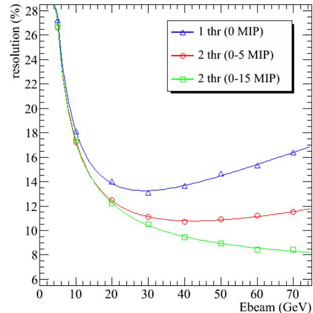
The response of a DHCAL is saturated (cell size VS  $R_M$ ) with consequences on the energy resolution.
