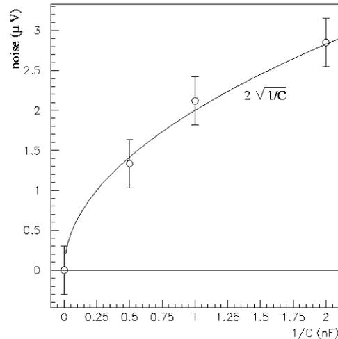
Measured  $kT/C$  noise versus  $1/C$ , compared to theoretical curve
