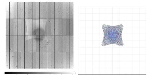
Internal reflexions between the  $g'$  filter and the surface of one lens of the Wide Field Corrector: MegaCam image (left) and ray-tracing simulation (right), reproducing the same 'pincushion' pattern. The ratio of surfaces explains why small reflexion coefficients yield a large effect (10%).
