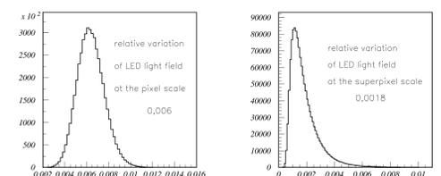
Stability of the LED illumination at each pixel/superpixel, evaluated on 16 successive shots in identical conditions.
