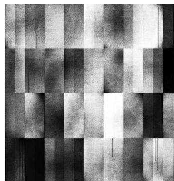
Illumination with a 850 nm LED, without filters (plotted for maximum contrast). The difference in responses at the level of the half-CCDs are due to the different gains of the readout amplifiers. The inhomogeneities of CCD efficiencies are also detected.
