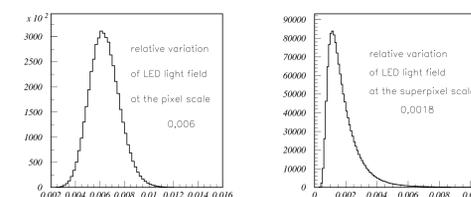
Stability of the LED illumination at each pixel/superpixel, evaluated on 16 successive shots in identical conditions.
