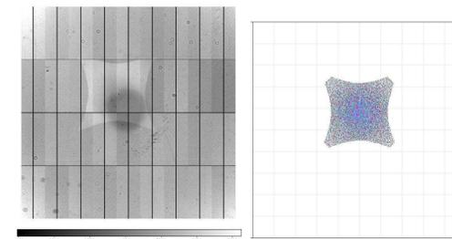
Internal reflexions between the  $g'$  filter and the surface of one lens of the Wide Field Corrector: MegaCam image (left) and ray-tracing simulation (right), reproducing the same 'pincushion' pattern. The ratio of surfaces explains why small reflexion coefficients yield a large effect (10%).
