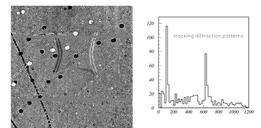
Tracking of diffraction pattern (left) when the illuminated spot is moved on the mirror. Four images have been stacked with alternate signs for visualization. The distances by which all features have moved are compiled in the plot on the left. The two prominent peaks mean that most of the optical faults are located in two optical planes, one being the mirror and one the front surface of the Wide Field Corrector.
