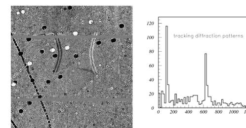
Tracking of diffraction pattern (left) when the illuminated spot is moved on the mirror. Four images have been stacked with alternate signs for visualization. The distances by which all features have moved are compiled in the plot on the left. The two prominent peaks mean that most of the optical faults are located in two optical planes, one being the mirror and one the front surface of the Wide Field Corrector.
