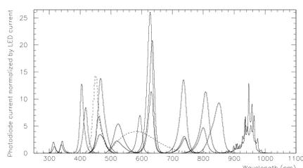
Spectra of the 24 LEDs selected for the calibrated LED source, and of the 'white' LED used for the artificial planet (dashed line).
