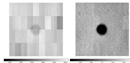
A 480 nm LED illuminating the mosaic with the filter  $g'$  in front of the CCDs (left). By making the ratio of that image with one taken without any filter, we obtain the  $g'$  filter transmission (right), showing an inefficiency of 10% in the center.
