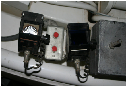
Picture of the current continuum lamps available at the Mayall “low flux” lamps have a blue filter to balance their spectrum.
