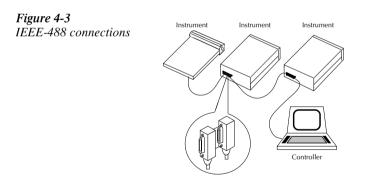
To avoid possible mechanical damage, stack no more than three connectors on any one unit.
