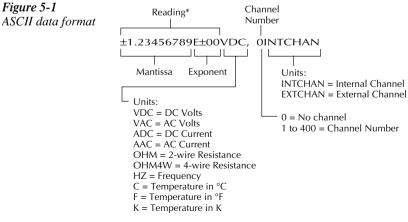
\* An overflow reading is displayed as +9.9E37 with no units
