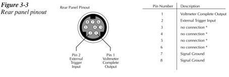
\* Either pin 3 or 5 may be configured as an output instead of pin 1. Either pin 4 or 6 may be configured as an input instead of pin 2. See the optional Model 2000 Repair Manual for details.
