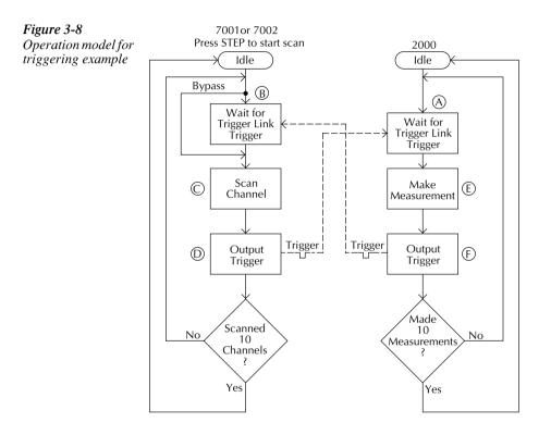
A Pressing EXT TRIG then STEP or SCAN on the multimeter places it at point A in the flowchart, where it is waiting for an external trigger.
