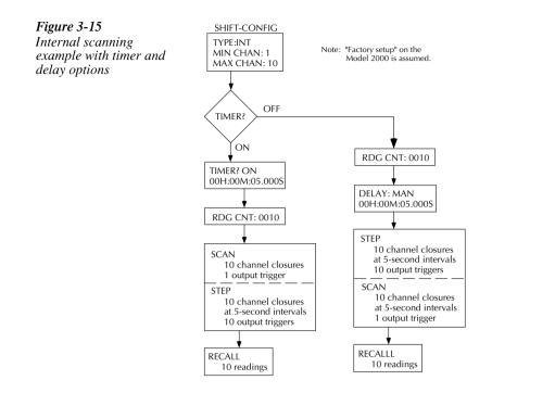
When using both the timer and delay parameters, the timer is not started until after the delay. For example, if the timer is two minutes and the delay is ten seconds, the timer is not started until 10sec after pressing SCAN. Each successive scan will occur at 2:10.0, 4:10.0, etc.
