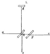
reflected to the mirror d. The mirrors c and d were of plane glass, and silvered on the front surface. From these the light was reflected to b, where the one was reflected and the other refracted, the two coinciding along be.
