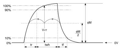
Note) Readout clock is used by composing vertical transfer clocks V $\phi$ 2A and V $\phi$ 2B.
