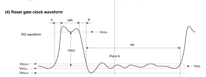
VRGLH is the maximum value and VRGLL is the minimum value of the coupling waveform during the period from Point A in the above diagram until the rising edge of RG.
