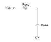
Reset gate clock equivalent circuit
