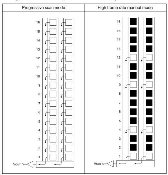
**Note)** Blacked out portions in the diagram indicate pixels which are not read out. Output starts from the line 1 in high frame rate readout mode.
