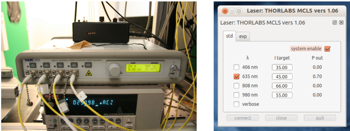
Figure 2: ThorLabs lasers. On the left, the Thorlabs box with its frontend and the fibers connected on the four outputs. On the right, the C++/Qt GUI to control it.
