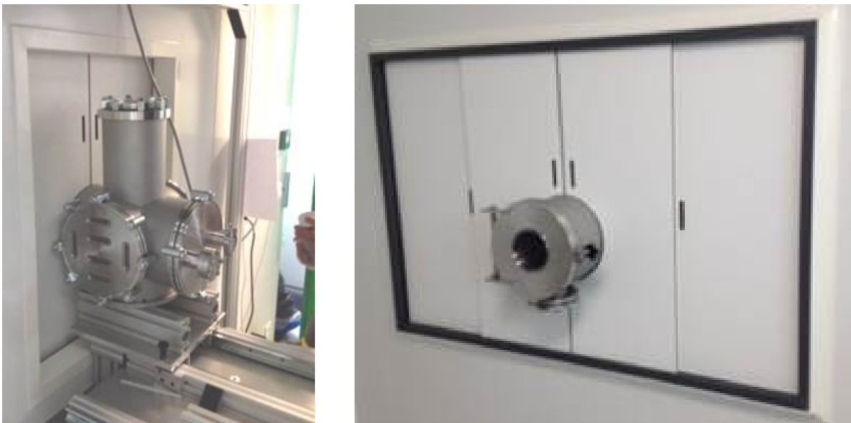
Figure 2.1: The “guillotine” door connecting to the class 10000/ISO-6 room for CCD loading/unloading. Left: seen from the testbench room. Right: seen from the class 10000/ISO-6 room.
